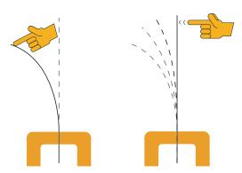
**Elastic Distortion:** The panel comes back to its original shape when the tension is released.
