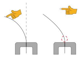
Plastic Distortion: The panel stays in the damaged shape even if the tension is released.
