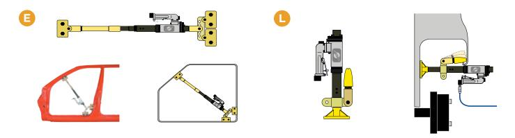
Set clamps at an angle to pull the corner of a door frame.
