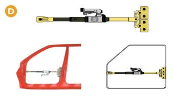
Using two wide clamps on one side allows you to carry out intensive pulling or pushing.
