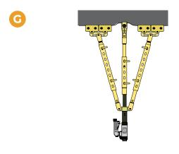
Very useful to pull a sill panel as you can spread the load onto the panel and pull only the desired part.
