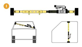
Grooved feet prevents damage to the panel edge.
