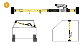
Grooved feet prevents damage to the panel edge.
