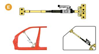
Set clamps at an angle to pull the corner of a door frame.
