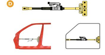
Using two wide clamps on one side allows you to carry out intensive pulling or pushing.
