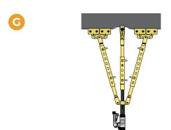
Very useful to pull a sill panel as you can spread the load onto the panel and pull only the desired part.
