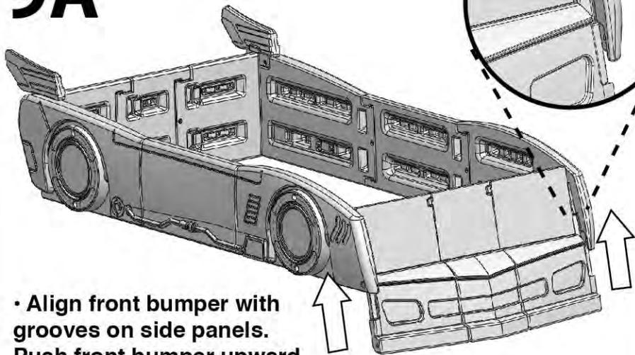
• Align front bumper with grooves on side panels. Push front bumper upward into a fully locked position.
