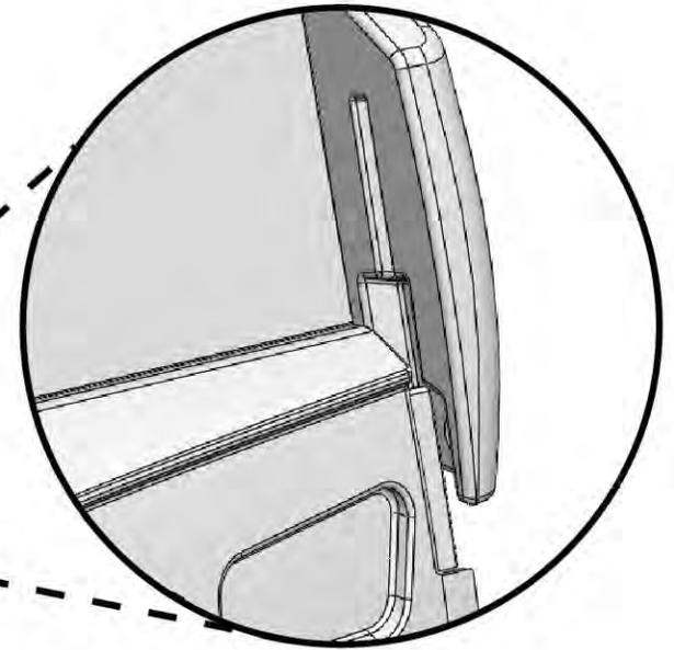
• Align front bumper with grooves on side panels. Push front bumper upward into a fully locked position.
