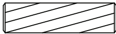
KK. M8x30mm Wood Dowel x2 Cheville en Bois M8x30mm Pasador de Madera M8x30mm
