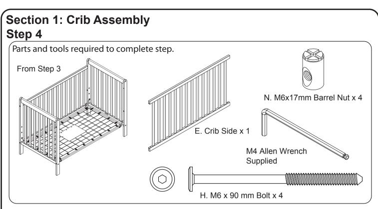
Attach (1) Crib Side (Part E) to the assembly from step 3 using (4) M6x90mm Bolts (Part H) and (4) M6x17mm Barrel Nuts (Part N). Tighten with the M4 Allen Wrench. Use the Flat Head Screwdriver to hold the Barrel Nut in the proper alignment.
