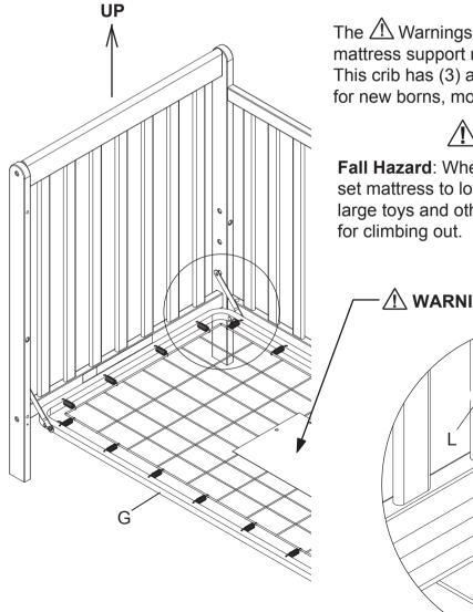
The A Warnings printed on the pouch attached to the mattress support must face up, the springs must face up. This crib has (3) adjustment positions, use the highest only for new borns, move the mattress down as the child grows.
