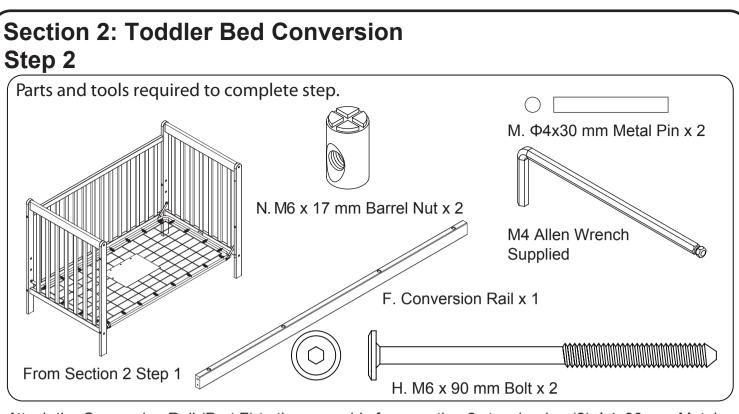
Attach the Conversion Rail (Part F) to the assembly from section 2 step 1 using (2) Φ4x30 mm Metal Pins (Part M), (2) M6x90mm Bolts (Part H) and (2) M6x17mm Barrel Nuts (Part N). Tighten with the M4 Allen Wrench. Use the Flat Head Screwdriver to hold the Barrel Nut in the proper alignment.
