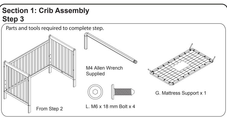
Attach the Mattress Support (Part G) in all corners using (1) M6x18 mm Bolt (Part L) in each corner. Tighten with the M4 Allen Wrench.
