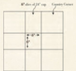
Cap for 26" Pier: Size: 30" square Note: Leave 6" square in center open for plantings or cover with 24" pier cap.
