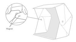
2 Install the backdrop inside the Foldio3. Take note that the backdrop installation is different depending on the color of the backdrop.
