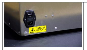
Step 1 – Ensure the power switch is set to off (0).
