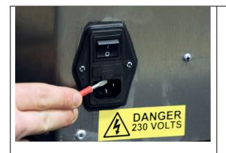
The iMelt system fuse is integrated within the IEC power socket. Exact models may vary.
