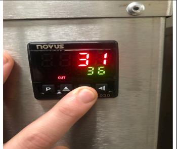
Use the up and down arrows to adjust the SV (green) to the desired temperature.
