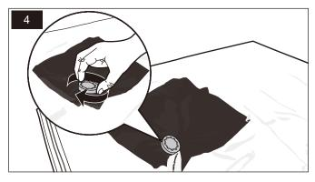
Tighten the white cap after vacuuming (Fig. 4).
