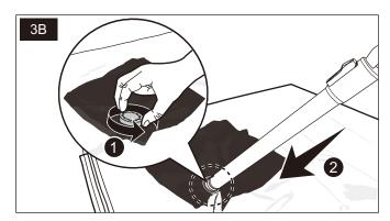
Remove the white cap and vacuum the air using the hand pump (Fig. 3a) or a vacuum cleaner (Fig.3b).
