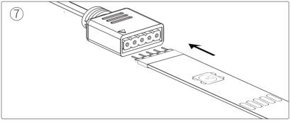
The 5V 2A power supply of the Controller unit PLUS can only support 2 meter light strip for 60 LEDs/m or 4 meter light strip for 30 LEDs/m. If there are more light strips, please connect them together and provide additional power with power supply line.
