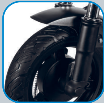
10 Inch honeycomb tubeless tyres.
