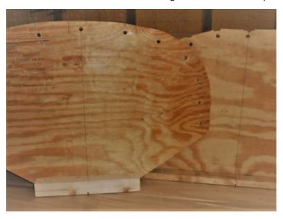
Note the reference lines and notches on the stations and the use of  $1 \times 2$  and  $2 \times 2$  cleats.
