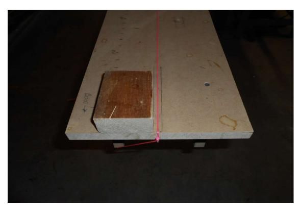
Clamp the stem to the cleat, check to make sure the string runs down the center of the stem, check for square and shim if necessary (note the small white paper shim between the block and the stem in the picture below.) The boat in this picture is mostly finished but it shows that you'll be using this block attachment throughout the build, so do it right at the beginning.
