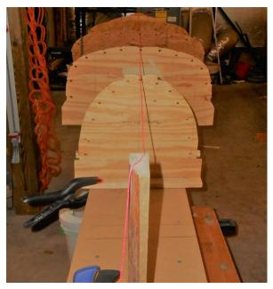
At this point, the stations should be perfectly aligned on the strongback because the notches are straddling the wire, and the edge of the station matches the square line. However, the top of the stations (where the keelson will be installed) must also be checked. Any twist in the strongback or variance in cutting and building the stations will be obvious at this point.
