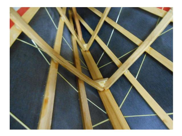
In this boat, you can see the last two ribs have been beveled to the keelson and to each other. They are then glued and reinforced with a small piece of ash from a cut rib. The second to last rib can normally be bent into this shape in a single piece. It may help to reduce the thickness of the rib in the middle where it contacts the keelson, which helps it to make the severe bend.
