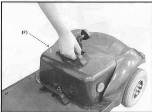
Figure 3. Use the battery pack handle (F) to pull the battery pack up and off the scooter. Batteries are heavy. When lifting please adopt the correct lifting posture to avoid injury. Ask for assistance if necessary.
