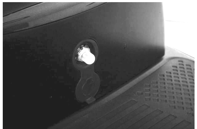
Battery box charging socket and circuit breaker reset
