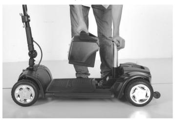
Locate the release lever as shown below. The lever is sprung, lift it to the vertical position 'A' and while holding the seat post lift the lever upwards 'B' and the two parts of the scooter will separate.
