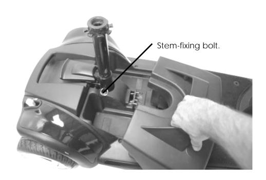
The higher the seat is adjusted; stability may be affected due to the higher centre of gravity.
