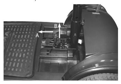
To reassemble tilt the rear part of the scooter backwards and locate the rear frame tube into the frame locating lugs (shown right). The scooter then should click back together. Lift the release lever to ensure that the locking relocates mechanism fully and that there is no debris fouling the mechanism.
