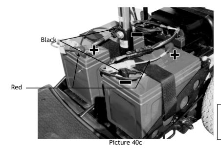
Picture 40c shows 70Ah batteries (optional extra) Scooter fitted with 50Ah as standard
