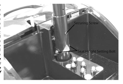
IMPORTANT: Your seat height is set in the lowest position for shipping purposes. In this position the seat must be removed to allow the battery pack to be removed.
