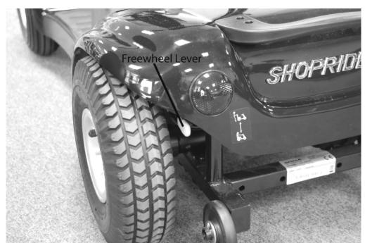
When in freewheel mode the scooter may be pushed at a walking pace. The scooter will 'auto-brake' if this speed is exceeded.
