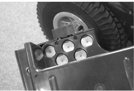
We also recommend that the connectors between the battery pack and the main chassis are also treated at the same time to prevent any carbon build up (round plate connectors and pins). Simply re-assemble the scooter as per user manual after these procedures have been undertaken.
