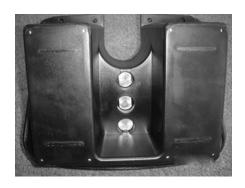
We also recommend that the connectors between the battery pack and the main chassis are also treated at the same time to prevent any carbon build up (round plate connectors and pins). Simply re-assemble the scooter as per user manual after these procedures have been undertaken.
