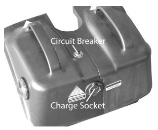
charged with the packs connected to the scooter or off board. Please make note of the comment above regarding the re-assembly of the pack if charging off board.
