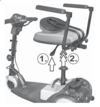
2.) Removing the battery case
