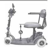
The seat height (h) is adjusted using the five holes (B1 - B5) in the seat support.
