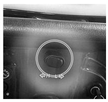
Move the toggle switch to setting  $\mathbf{H}$  or  $\mathbf{L}$  to adjust the required maximum driving speed.
