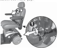
Lift the seat while pulling the seat lock (3) out of the seat support (4).
