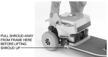
FIGURE 14. REMOVING THE REAR SHROUD
