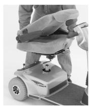
FIGURE 13. REMOVING THE SEAT
