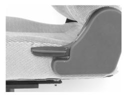
FIGURE 10A. SEATBACK ADJUSTMENT LEVER
