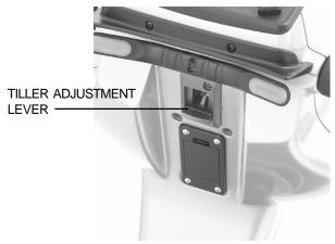
FIGURE 9A. TILLER ADJUSTMENT
