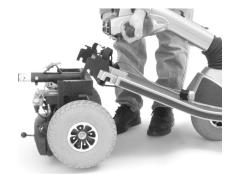
FIGURE 20. SEPARATING THE FRAME SECTIONS
