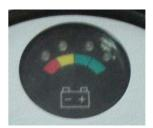
The remaining power indicated by the battery gauge will vary by the driving time incurred and how you drive. Repeated starting, stopping and climbing will consume power more quickly. The gauge is shown below.
