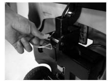
2. Lift up the scooter and then reinsert the locking pin. Slowly lower the front of the scooter.
