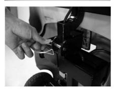
4. Push the front of the frame slightly to take the pressure off the pin, then remove the locking pin from the frame.
