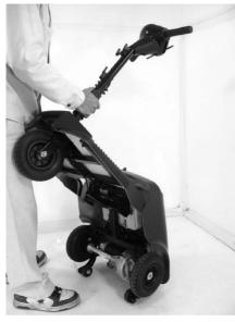
5. Lower the front section and then the two sections can be detached.
