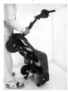
1.Stand the rear section up and insert the front section in to the receiver.
