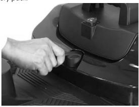
3. Then lift out of the scooter using the handle on the battery pack.
