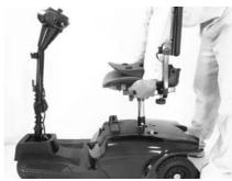
4. Replace the seat and rotate it until it locks in to its correct position.
