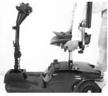
1. Push the Seat Rotate Lever whilst pulling up on the seat to remove.
