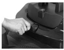
3. Lower battery pack in to the compartment in the scooter and then turn the handle to secure the pack in place.
