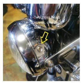
Gently pull the lens and reflector off (very tight) make sure you do not damage the cable connection. Cable is threaded through a hole in rear of headlamp housing
