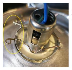
Remove rubber cover over existing bulb connector and retain for refitting. Release existing bulb and cable by pressing clip ends together. Lay aside bulb, bulb holder and cable loom (no longer required). Retain the spring clip.
