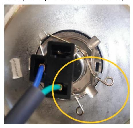
Refit lens and headlight back in place using two larger chrome cross head screws and check head light works correctly.
