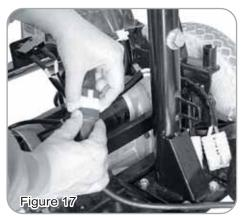
Release two Guide Pins to separate Front and Rear Sections. (See Fig. 18) With one hand on rear frame and other on seat post as handheld, detach Front and Rear Sections. (See Fig. 19)
