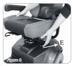
Attach Front Basket. Adjust Seat Height: If the seat height is not correct, remove seat from scooter. Use a screwdriver to raise or lower the seat. Remount seat on seat post. Adjust Tiller Angle position: Use the Tiller Angle Adjustment Lever to adjust the tiller to a comfortable position.
