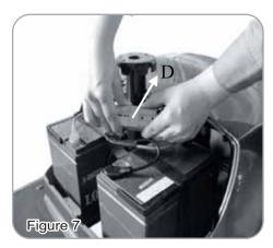
Place battery cover over batteries.(See Fig. 8)
