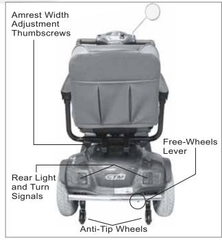
Figure 3 - HS-740 Scooter Rear View
