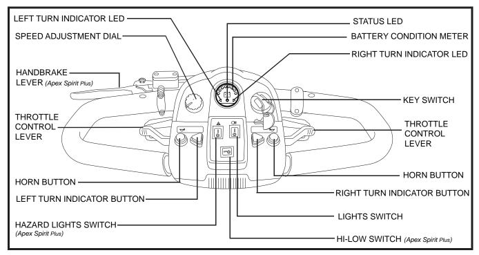
**Figure 4. Tiller Console Components**
