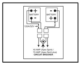
Figure 11. Battery Wiring Diagram
