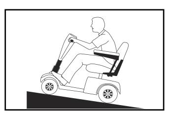
Figure 2A. Increased Stability Driving Position
