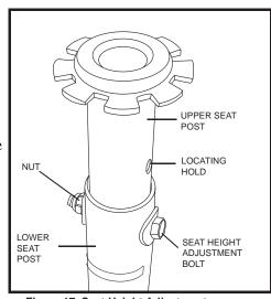
Figure 17. Seat Height Adjustment
