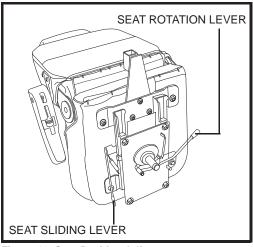
Figure 16. Seat Position Adjustments
