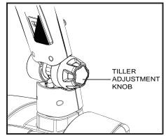
Figure 12. Tiller Angle Adjustment Knob
