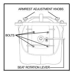
Figure 15. Seat Adjustments
