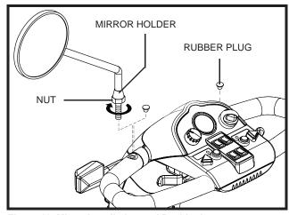
Figure 13. Mirror Installation and Positioning
