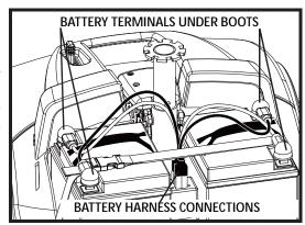
Figure 10. Battery Removal/Installation
