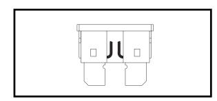
Figure 18A. Blown Fuse (Replace)
