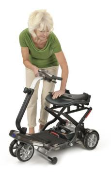
4. Finally push the tiller against the seat and the front of the floor pan towards the rear wheels to ensure your Minimo is locked into the folded position.
