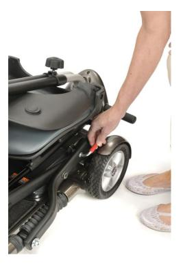
2. Pull the tiller away from the floor pan until the front wheels of your Minimo touch the floor.
