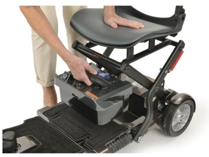
To remove the battery pack of your Minimo first ensure the pack is unlocked by inserting the key into the pack and turning it 90° anti clockwise to the unlock position. Then simply lift the pack up away from the base of the scooter and the seat using the handle provided.
