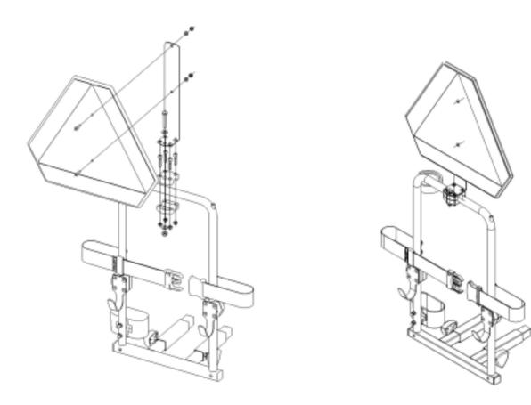
• Position the rear reflector as shown in the drawing.
