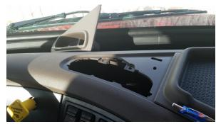
Remove plastic panels on vehicle dash using nylon pry bar. There will be 2 in total.
