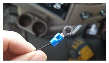
Crimp a ring terminal to the black/ ground wire on the GPS unit harness
