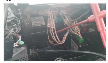
Locate wires underneath the fuse box. You will be looking for a 12 volt constant source and a true ignition.
