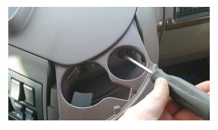
Pull out cup holder and remove the 2 screws holding it in place.
