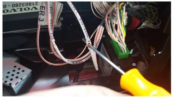
Use a pick tool to poke a hole through the wires.
