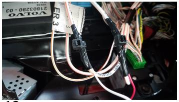
Tape connections with electrical tape. Then secure the connection with a zip-tie directly over where you spliced into the wires.
