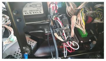
Put a zip-tie over any fuse holders (if applicable) to prevent tampering and to clean up harness. Bundle up wiring harness and secure it. Make sure there is no stress on your wiring connections!
