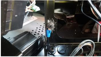
Find a good chassis ground (Metal connected to the vehicle body/frame) and sand down the area if any paint is present. Use a self-tapping screw to make the connection/ Alternatively, you may use an existing bolt or ground wire.
