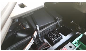
Mount the GPS device high up in the dash, and ensure it is free of any metal obstructions (this can interfere with the GPS/cellular signals) Use zip-ties or similar method to secure the device. Now all that's left to do is test your device and re-assemble the vehicle dash!
