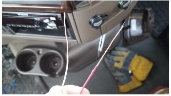
Prepare the wires on the GPS harness for connection by stripping back the insulation 2-3 inches and twisting tightly.
