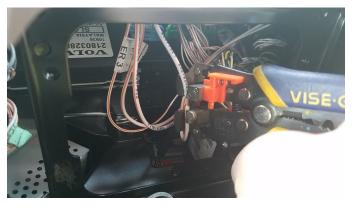
Using an automatic wire stripping tool, take back the insulation on the wires you will be connecting to. Take care not to short-out any of the exposed wire to a metal surface.
