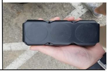
3. Attach to the underside of vehicle/asset. We recommend using the frame rail or bumper if possible. Make sure to keep away from moving parts and exhaust pieces!
