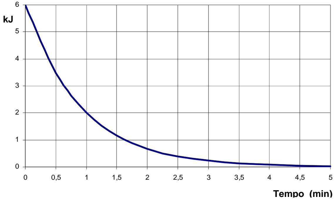
**COOLING CURVE OF TUBE HOUSING ASSEMBLY**
