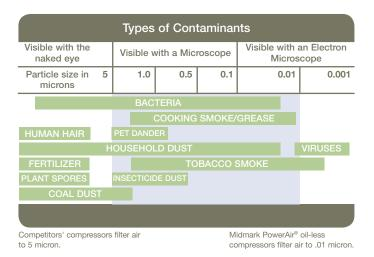
Contaminants that pass through a 5 micron filter
