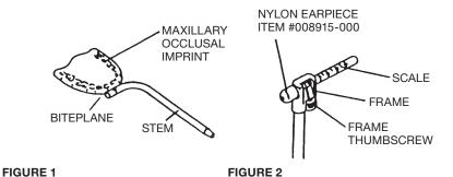
3. Slightly unturn the two frame thumbscrews and slide the scales outward to abut the nylon earpieces with the frames, Figure 2. The nylon earpieces are threaded onto the scales and may be removed for cold sterilization.
