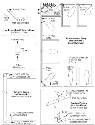
The vacuum lines should be supported to prevent sag and should be sloped 1/4 inch (6 mm) for every 10 feet (3m) towards the vacuum pump.
