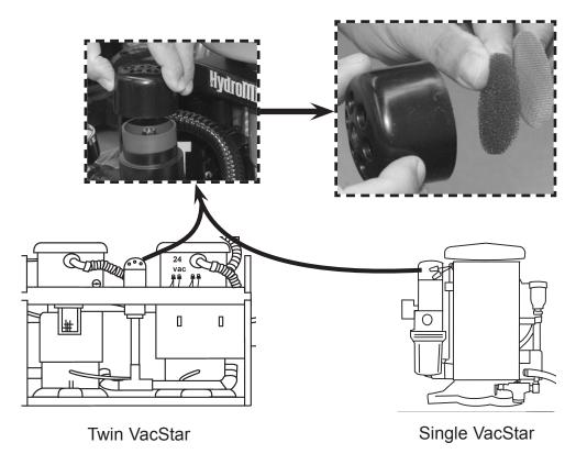
Figure 11. Vacuum Relief Valve Filter Location
