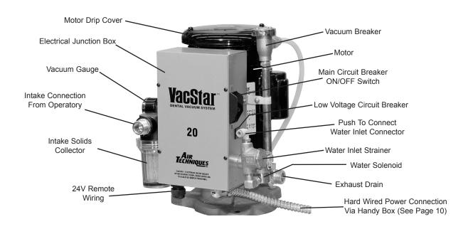
Figure 1. VacStar 20 and 40 Parts Location
