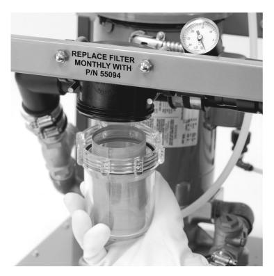
Figure 12. Intake Solids Collector Location
