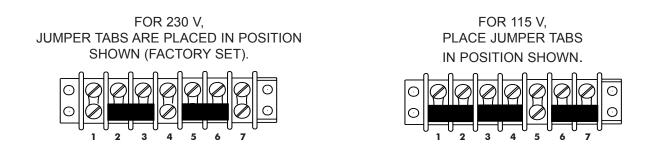
Figure 9. VacStar Electrical Junction Box - Interior View VacStar 20 (Factory Set for 230 V)
