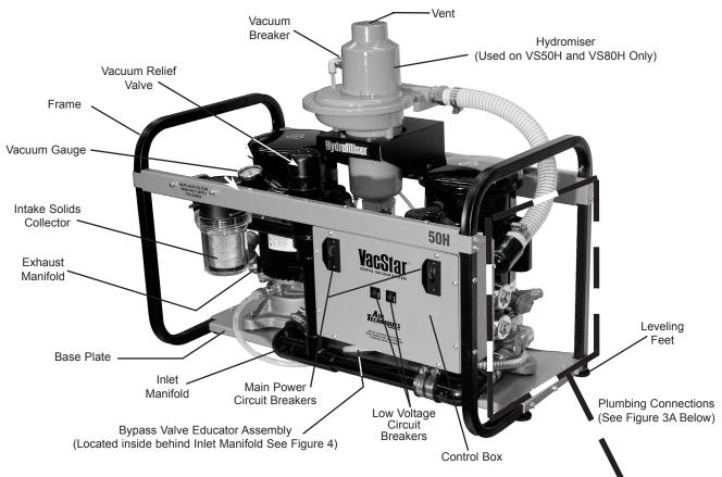
Figure 2. VacStar 50, 50H, 80 and 80H Parts Location NOTE: VACSTAR 50H Shown, Other Models are Similar
