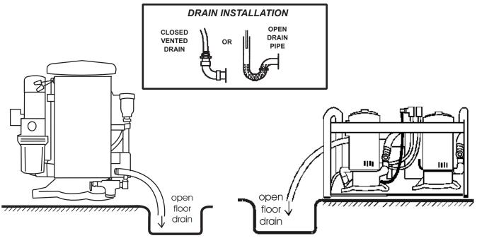
Figure 4. VacStar 20, 40 without a HydroMiser or Air/Water Separator
