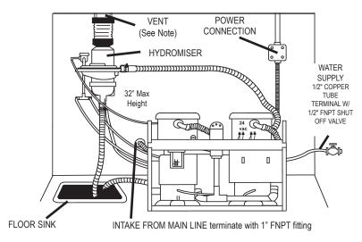
Figure 8. VacStar with Wall-Mounted HydroMiser
