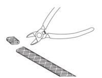
**STEP 2:** Push the braid back 2 inches from the cable end.
