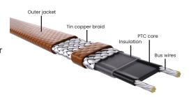
The extruded core tape, which made by parallel tinner copper bus wire and PTC semiconductor polymer heating material, and inner insulation layer of fluoropolymer are added to tinned copper braid and the outer jacket form a complete structure of MVM heating cable, in which the outer jacket can be made of fluoropolymer material (CT).
