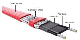
The extruded core tape, which made by parallel tinner copper bus wire and PTC semiconductor polymer heating material, and inner insulation layer of fluoropolymer are added to tinned copper braid and the outer jacket form a complete structure of MVH heating cable, in which the outer jacket can be made of fluoropolymer material.
