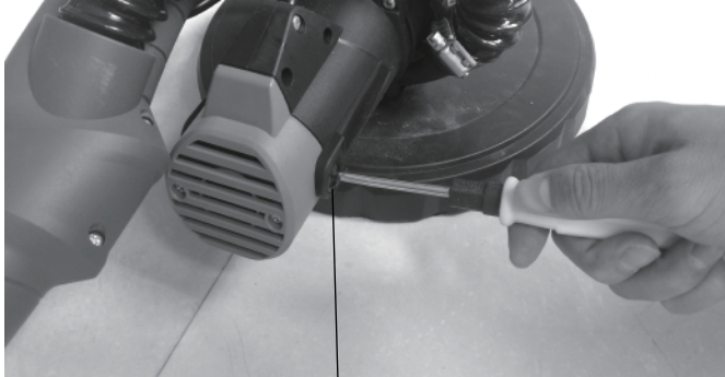
Position to replace the carbon brushes
