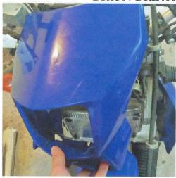
1) Remove the stock headlight cowling.(3 screws, 1 on each side, and 1 in the center under the headlight)
