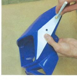
2) Use the provided hole pattern to mark holes on your stock shroud for drilling.
