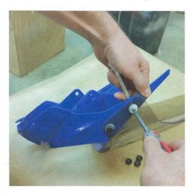
5) Tighten all 4 screws using a Phillips head screwdriver and an 8mm wrench. (Do not over tighten)
