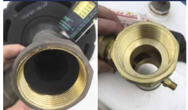
Unblock Tank Vent Filters of Air Pollution (Dust and Water mix with Fuel)
