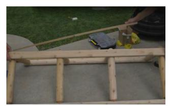
Locate the roof peak boards. (Angled cut side)
