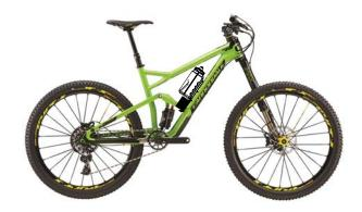
FS MTB frames with rocker positioned across frame triangle.
