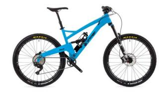
FS MTB frames with shock mounted across frame triangle.
