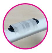
For non uniform and narrow tubes we advise to hold in place with tape whilst curing.
