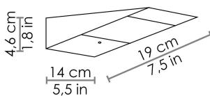
Wall lamps in dark grey painted die-cast aluminium, with a polycarbonate diffusor. The high IP rating (IP54) makes the lamps ideal for indoor and outdoor use. The lamps are fitted with a solar panel that auto-charges the battery, a dusk sensor and a motion sensor (this solar product requires no electrical connection). Replac eable battery.
