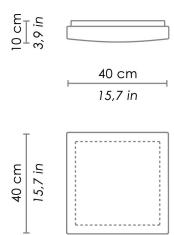
Wall-ceiling lamps with diffuser in mouth-blown, satin-finish opal triplex glass; matt white painted metal frame. The product is suitable for indoor use only.
