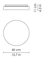
Wall-ceiling lamps with diffuser in mouth-blown, satin-finish opal triplex glass; chlorine-resistant, anti-UV, neutral translucent polycarbonate frame, with chrome or matt white painted metal parts. Twist-lock coupling system f or the glass component. The product is suitable for indoor use only. Drum Metal is IP44
