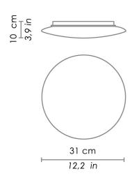
Wall-ceiling lamps with diffuser in mouth-blown, satin-finish opal triplex glass; chlorine-resistant, anti-UV, neutral translucent polycarbonate frame. Twist-lock system for the glass component. The product is suitable for indoor use only. IP44 rating.
