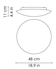
Wall-ceiling lamps with diffuser in mouth-blown, satin-finish opal triplex glass; white painted metal frame. Twist-lock system for the glass component. The product is suitable for indoor use only.
