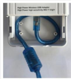
3. Replace the cover back onto the bottom of the antenna and make sure the wire is coming out of one of the holes on the bottom, so the unit is water tight.
