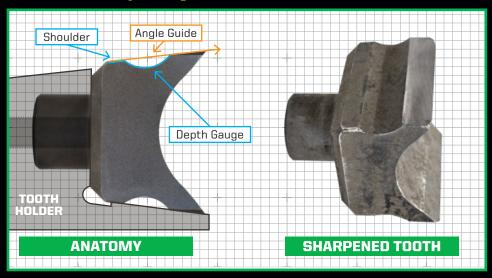
**Teeth can be sharpened while on your drum mulcher.** To do this, lightly sharpen the outside leading edge of each tooth with a  $4 \frac{1}{2}$ " angle grinder, equipped with a flap-style sanding disc. Use the shoulder, located behind the depth gauge, as an angle guide. Try to keep the angle the same on the front of the tooth as the back when you sharpen. Avoid touching the shoulder with your grinder. The shoulder needs to stay square so the tooth seats against the holder when you rotate.
